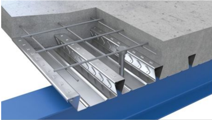
Figure 11: Composite metal deck detail
